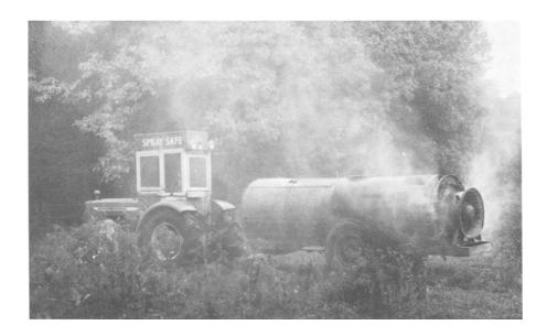
Fig. 2.-Equipment used to evaluate the air filtering-pressurization unit. Note: Spray clouds drifting forward over tractor cab and air filtering unit.
